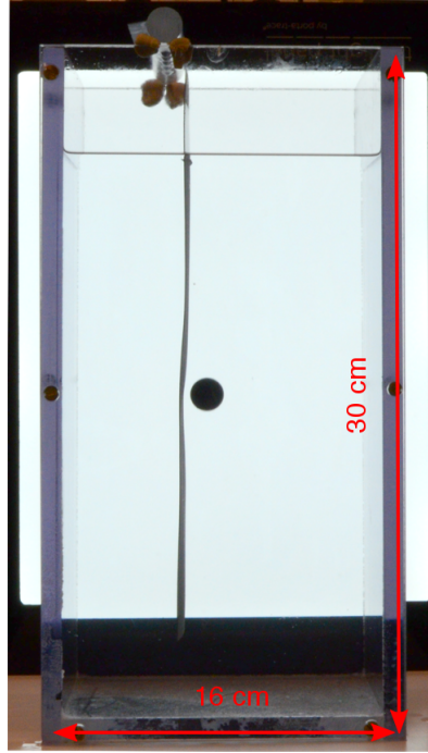
FIG. S1. Experimental setup: silicone rubber sheets of size 8 cm \times 30 cm are suspended in silicone oil (viscosity 1 Pa·s) in a glass tank of dimensions 16 cm \times 16 cm \times 30 cm. The immersed length of the sheet is 20 cm. The sheet is suspended under gravity with its top end held on a cylindrical rod and its bottom end free.
